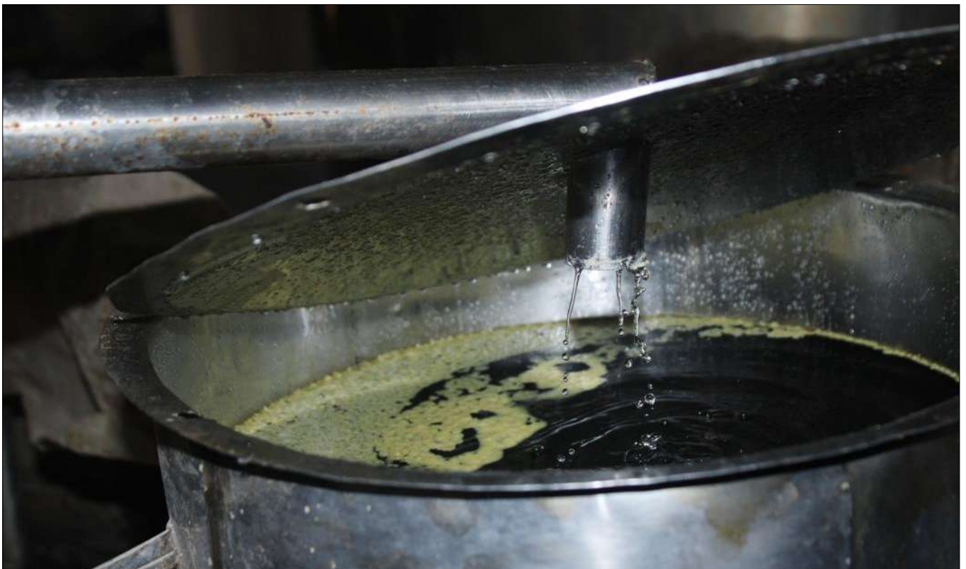
Freshly produced oil in collection drum of a distillation chamber
